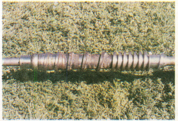
Fig. 11. Short pitched screw configuration.
