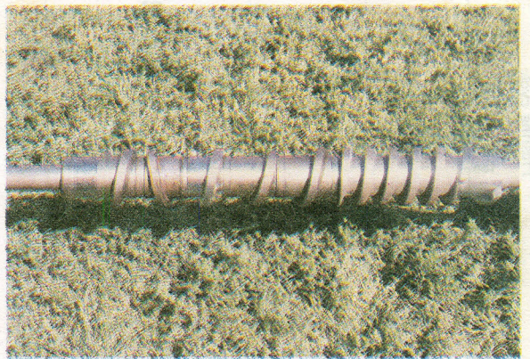
Fig. 12. Short pitched (3.8 cm) screw configuration.
