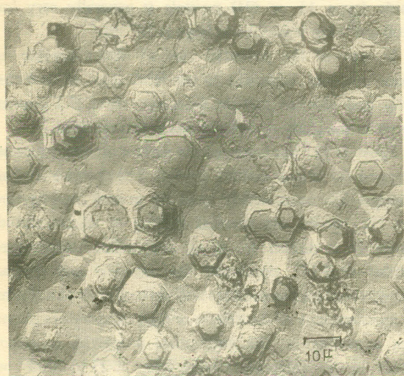
Fig. 1. Etch pits on (0001) plane. Crystal etched at 2500°, for 10 minutes.
