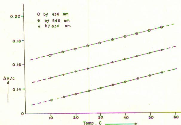
Fig. 1.  $\Delta n/c$  versus temperature for 0.06% conc.
