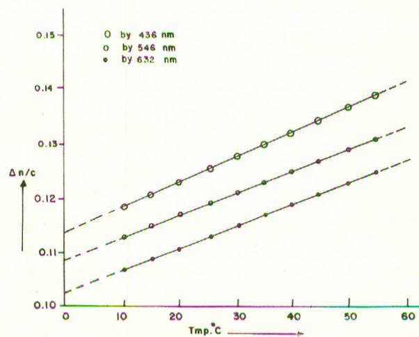
Fig. 2.  $\Delta n/c$  versus temperature for conc. 0.60%.
