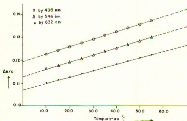
Fig. 3.  $\Delta n/c$  versus temperature for conc. 1.61%.
