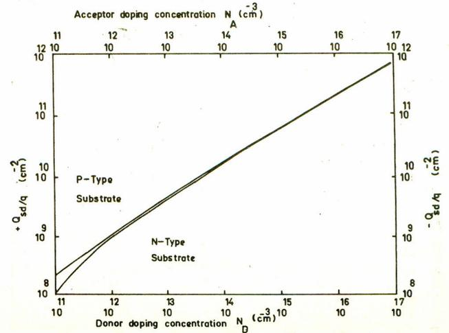
Fig. 4. The charge per unit area in the depletion region versus impurity doping concentration.
