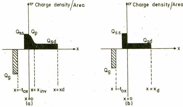
Fig. 2. Schematic diagram of charge distribution in a p-channel MOS field-effect transistor: (a) after inversion; (b) before inversion,  $Q_{sd}$  positive charge density;  $Q_g$  negative charge density.
