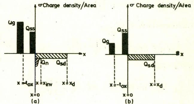
Fig. 1. Schematic diagram of charge distribution in an n-channel MOS field-effect transistor: (a) after inversion; (b) before inversion. ■ positive charge density; ▨ negative charge density.
