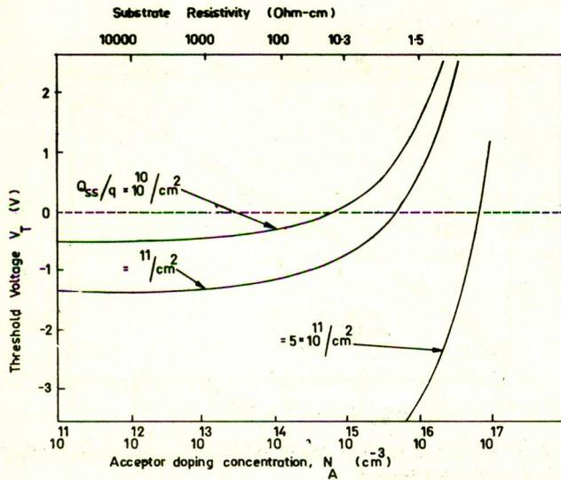
Fig. 6. Calculated theoretical threshold voltages for an n-channel MOS field-effect transistor with  $t_{ox} = 2000 \text{ \AA}$ .
