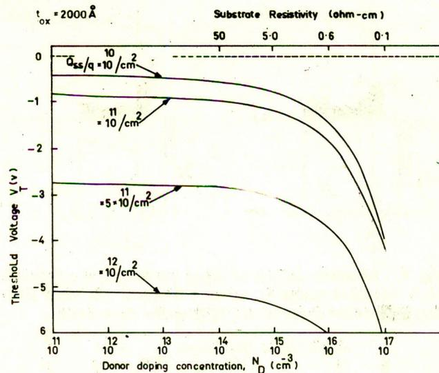
Fig. 8. Calculated theoretical threshold voltages for a p-channel MOS field-effect transistor with  $t_{ox} = 1000 \text{ \AA}$ .
