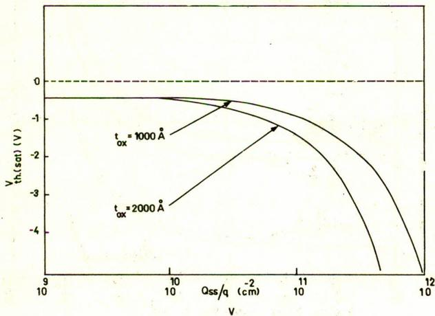
Fig. 7. Calculated theoretical threshold voltage  $V_{th}(\text{Sat.})$  versus charge carriers  $Q_{ss}/q$  on high resistivity.
