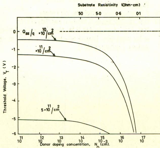
Fig. 9. Calculated theoretical threshold voltages for a p-channel MOS field-effect transistor with  $t_{ox} = 2000 \text{ \AA}$ .
