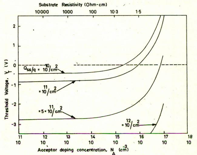
Fig. 5. Calculated theoretical threshold voltage for an n-channel MOS field-effect transistor with  $t_{ox} = 1000 \text{ \AA}$ .
