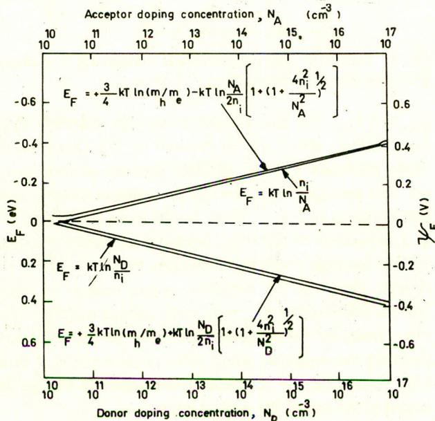
Fig. 3. Fermi potential as a function of impurity doping concentration.
