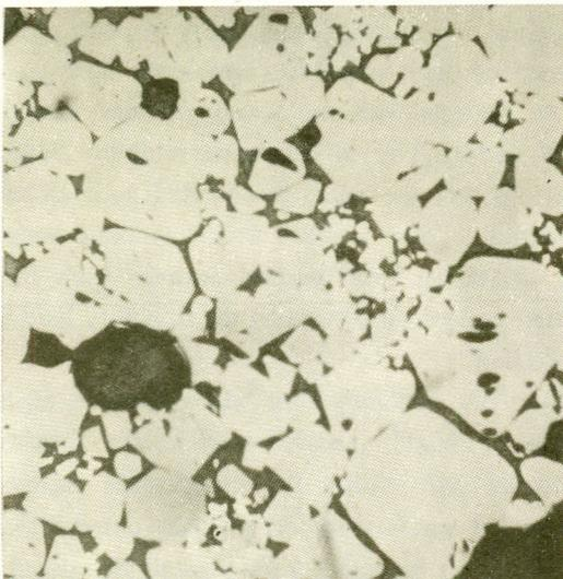
Plate 3. Micrograph ( $\times 400$ ) showing excess spinel. Spinel (angular bright crystals), periclase (big rounded grains), monticellite (light grey) and black spots are pores.
