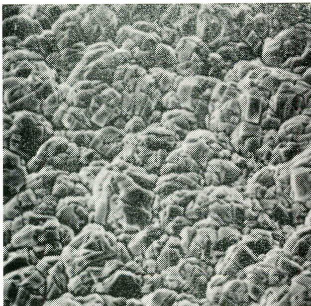
Fig. 2. SEM of freshly prepared \text{PbO}_2 on carbon, magnification, 3,000, 45^\circ .
