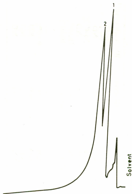
Fig. 1. Chromatogram of Anethum graveolens hydrocarbon run at 140° using PEGS column.
