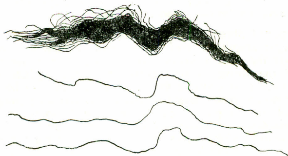
Fig. 2. Schematic diagram of medullated fibres withdrawn from staple exhibiting the secondary fibre crimp corresponding in varying degrees to the staple crimp.
