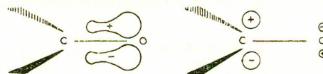
Fig. 1. Form of charge density in the ground (left) and excited states (right) of a carbonyl group.
