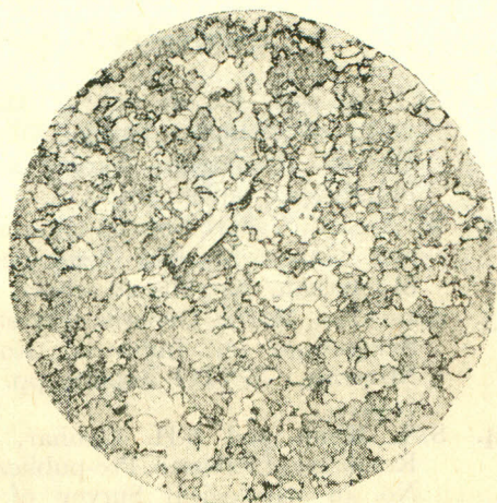
Fig. 5.—Photograph of dolomite showing Xenotopic texture. Grains are interlocked in a uniform mosaic. Muscovite flakes can also be seen. Magnification x (ordinary light).
