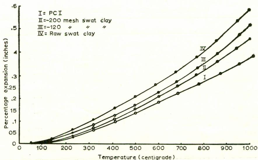
Fig. 2.—Reversible linear thermal expansion,
