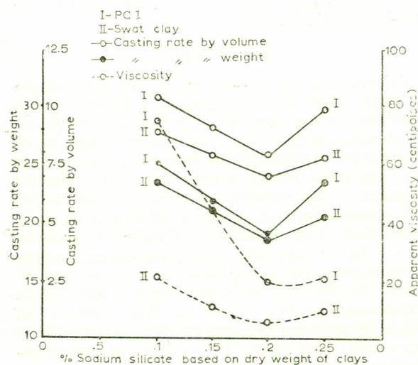
Fig. 3.—Viscosity and casting rate vs. amount of electrolyte.
