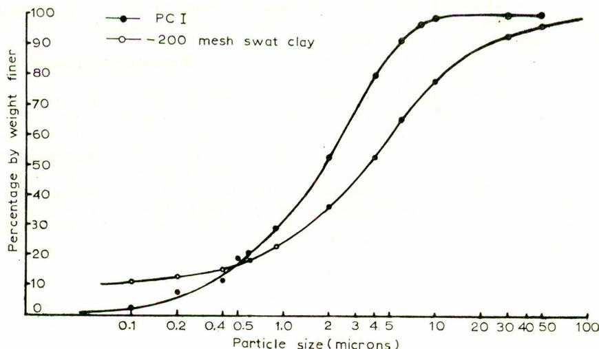
Fig. 1.—Sizing analysis (cumulative plot), logarithmic scale.
