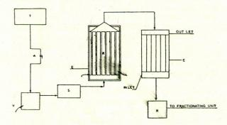
T, Alcohol feed tank; A, Feed control valve; V, Alcohol vapouriser; S, Electrically heated preheater; F, Temperature-controlled electric furnace; R, Ether reactor; C, Condenser; R, Receiver.
