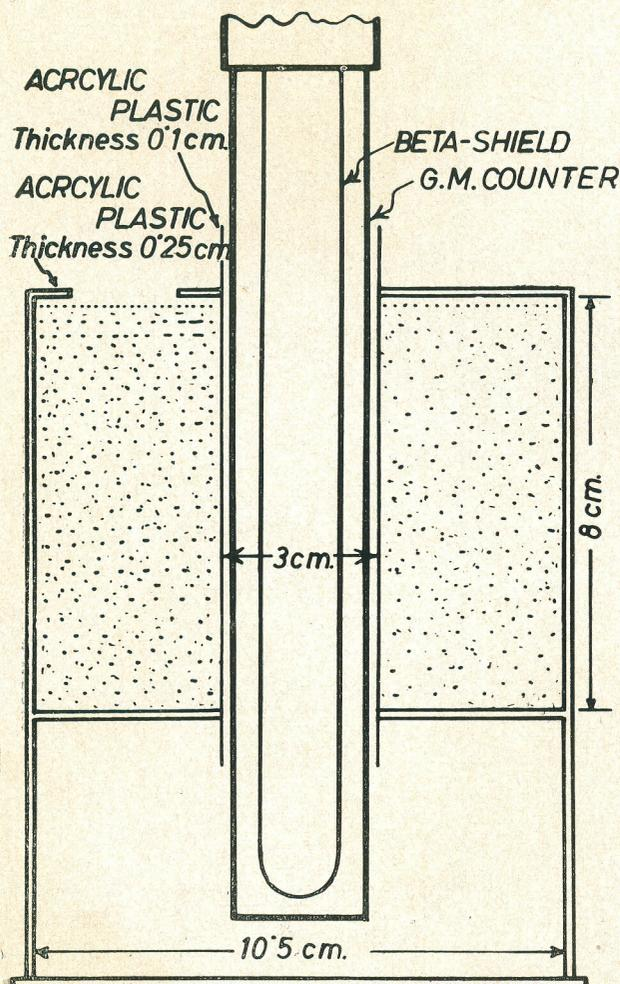
Fig. 2.—Cylindrical discriminator: diagrammatic sketch.
