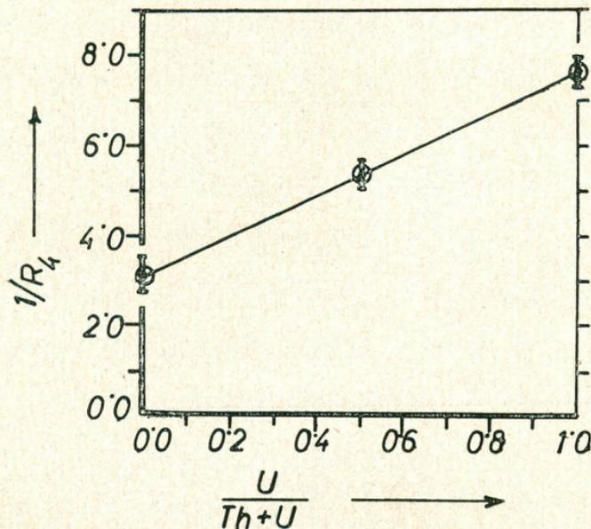
Fig. 3.—Graph showing the value of  $1/R_4$  for different ratios of uranium/(uranium + thorium) obtained with the cylindrical discriminator of Fig. 2.
