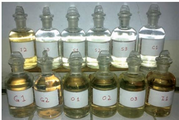
Fig. 3. Water samples collected from Basharat area near Hassan Kishor Coal Mine.
