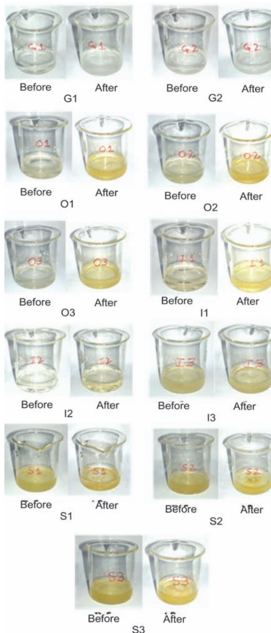
Fig. 4. Colour of the water samples before and after one day exposure to fresh air.
